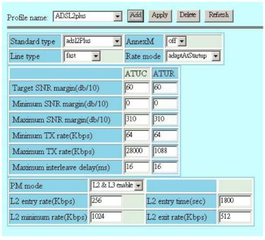
Figure 4-2 DSL Profile Configuration
